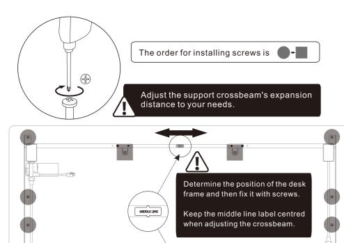
The distance from the support plate to the edge of the desktop should not exceed 200mm.
