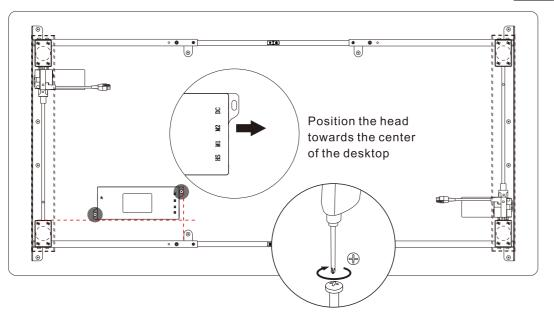
Please assemble the control box in accordance with the dotted line shown in the illustration. Please determine the control box's fixed position based on the length of the connecting cable.
