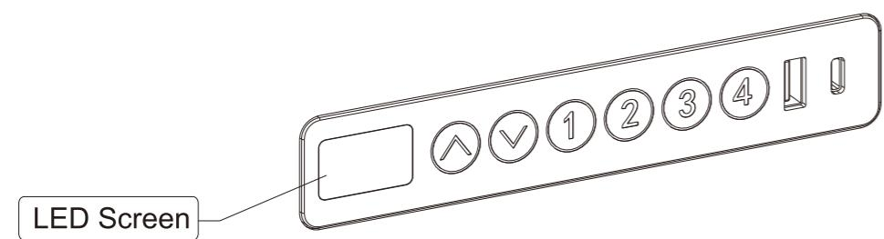
1. Press the up/down button to adjust the height of the desk. When the desktop runs to the lowest point, the screen will display "bot". Otherwise, the desktop will display "top" when the desktop runs to the highest point.
