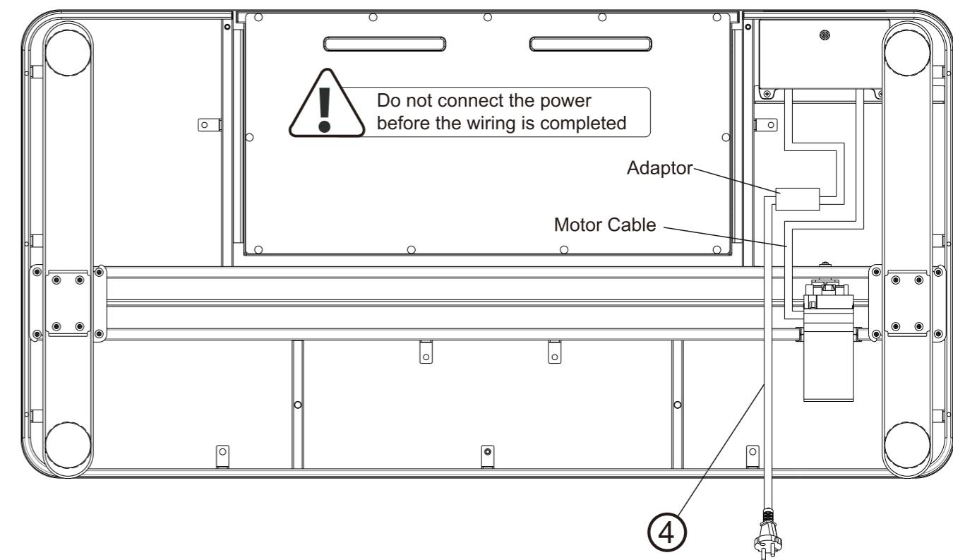
Fix the cables to the tabletop with cable tie(D) to keep desk clean.
