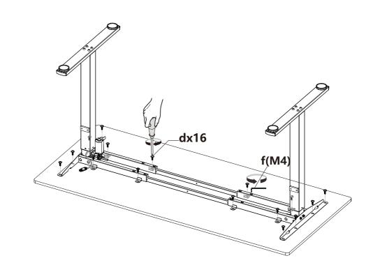
Note: Please pre-install 16 number "d"screws to the corresponding hole position, and then tighten them all in turn, finally use the "f(M4)"wrench to tighten the crossbar.
